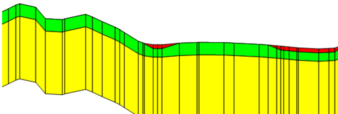
Figure 45: Example of vertical grid layout with a separate discontinuous layer (indicated in red) representing alluvial aquifers.
